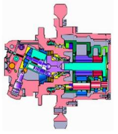
Travel reducers are ideal drives for wheeled or tracked vehicles and other mobile equipment. In addition, it can be applied wherever there is movement and rotation. Due to its particularly compact design, it can also be used in places where the installation environment is extremely difficult.
