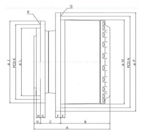
WR-WT series are designed for planetary type gear box of housing rotated application.
